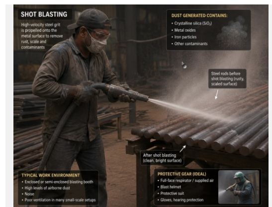
Fig. 3 – Shot blasting. High-velocity abrasive removes rust and scale from metal. Silica exposure depends on the abrasive and surface contamination; steel shot itself is not silica. Illustration from the case video.
